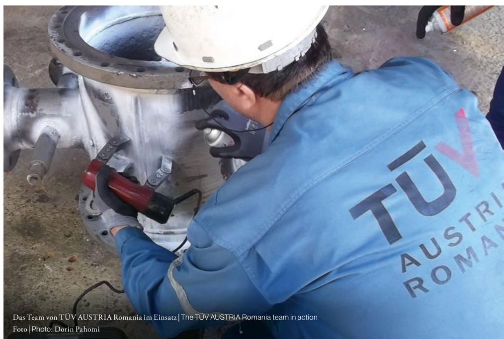
Schweißnähte unter professioneller Prüfung | Welding seams under professional examination Foto | Photo: Dorin Pahomi
